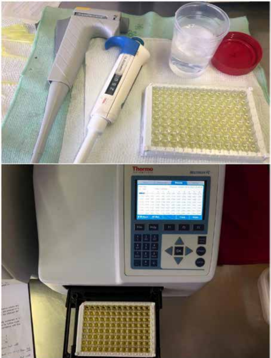
Figure 10 : ELISA procedure using microwells and micropipettes and ELISA reader to see results (photo by author 2021).
