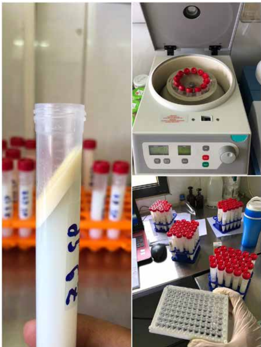
Fig. 9. Milk analysis after centrifugation and microwells for ELISA testing (photo by author 2021)
